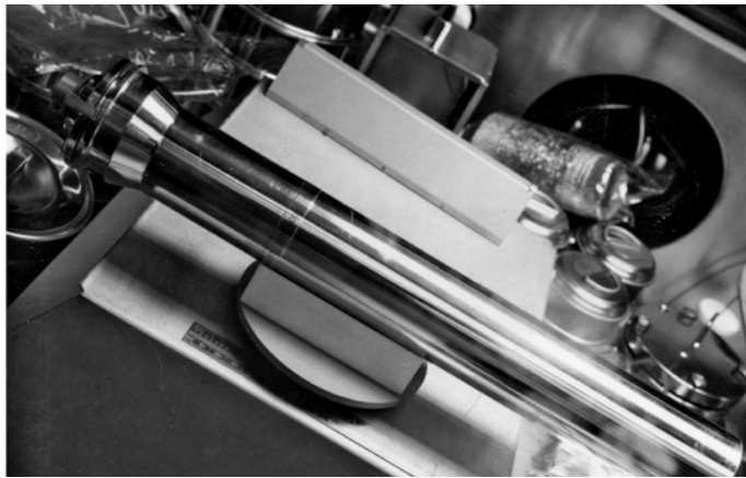
The Core Sample Vacuum Container (CSVC) holds an entire drive tube section. Apollo 16 and Apollo 17 astronauts collected one each. After the samples arrived at Johnson Space Center, the curators placed both CSVCs in an additional vacuum container with a much better seal. Both containers remain sealed in the center's Curation Storage Vault. They will remain there in pristine condition for future studies. NASA
