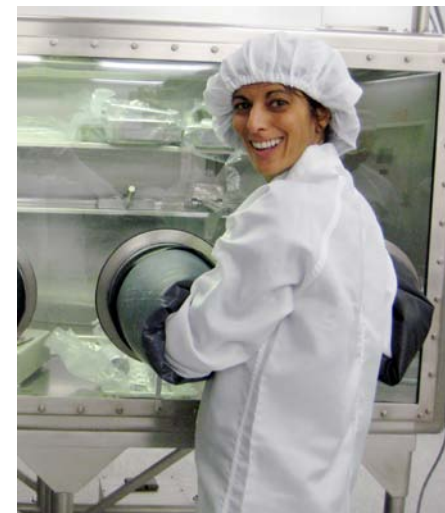
The author felt right at home in the Lunar Sample Laboratory. All sample handling is done inside glove boxes, such as the one shown here, that contain an atmosphere of clean, dry nitrogen.
