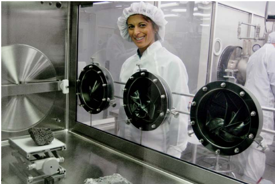
Researchers handle Moon rocks inside nitrogen-vented glove boxes in the Lunar Sample Laboratory.
