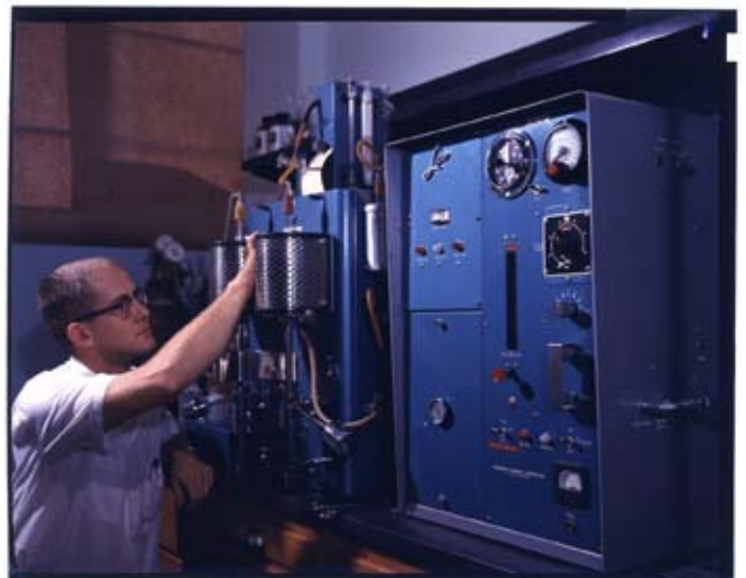
CMS Curator Charles Lewis analyzes a meteorite in the CMS's LECO carbon analyzer
